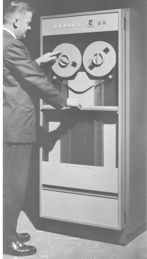
Model D 3030 magnetic tape units were designed by Datamec for medium speed computer market.
