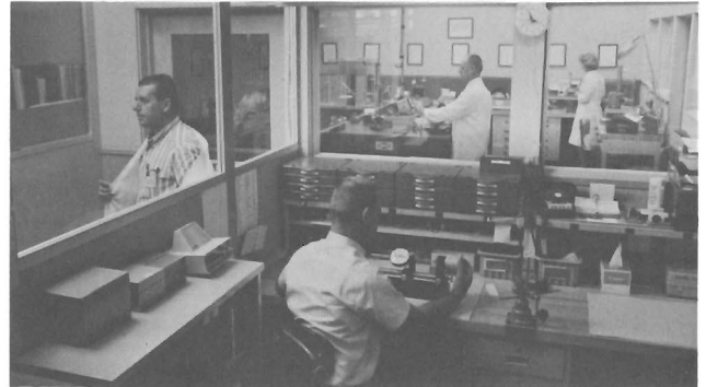
Overall view shows Hal Andrews in outer room calibrating a precision gage. Ralph Richberger, visiting from another department, dons white smock in air lock before entering "clean room" where precision calibration is done by Glenn Herreman and Irene Ardoin.
